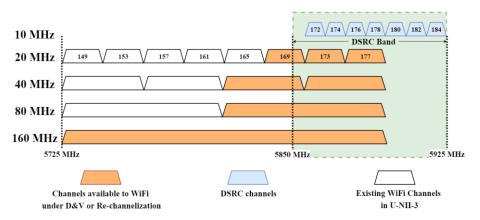
Figure 1 - An illustration of spectrum sharing in DSRC band
